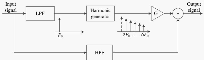
LPF: low-pass filter, HPF: high-pass filter, G: gain for generated harmonics
